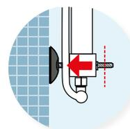
Fit the lift and the earthing terminal. Adjust the lower stop.
