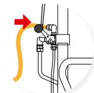
Fit the water connection to supply the circuit.
